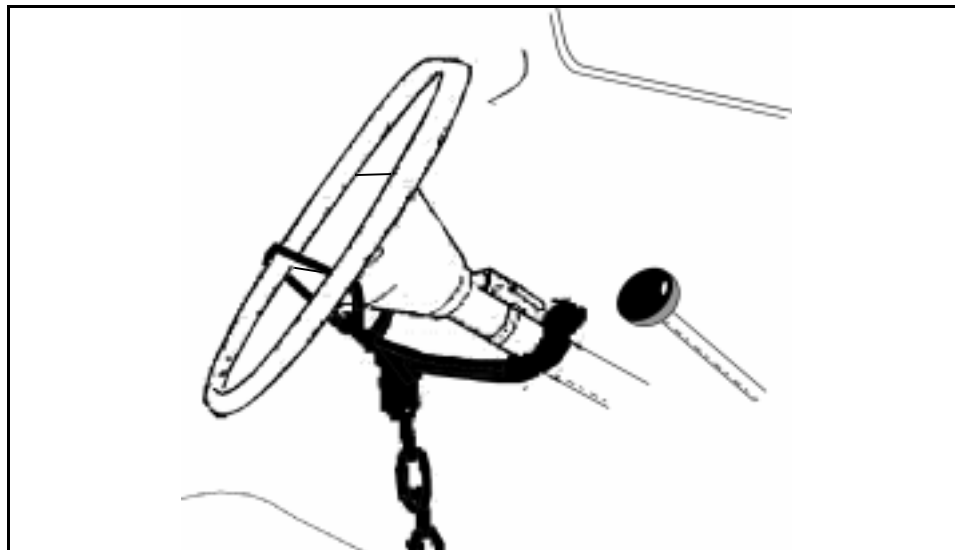
Figure B-7. Typical Clamp and Chain Installation
